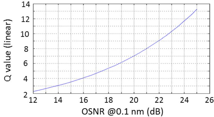
For  $L_A = 50$  km, from the graph  $Q \sim 7$ ; the BER is therefore  $\text{BER} \sim 1.3 \cdot 10^{-12}$
